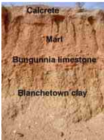
Blanchetown clay (as labelled) underlying Bungunnia limestone in a soil profile between Morgan and Swan Reach
